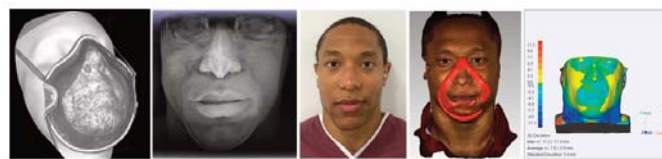
Figure 2: (L-R) MicroCT image of FFP3 mask on 3D head phantom. MRI scan of participant with corresponding photo of visible soft tissue deformation following MRI examination. Surface scan of participant with inner surface of mask, and registered scan showing effect of gravity on the soft tissue.
