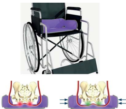
Figure 1: Schematic of the pressure equalisation device
